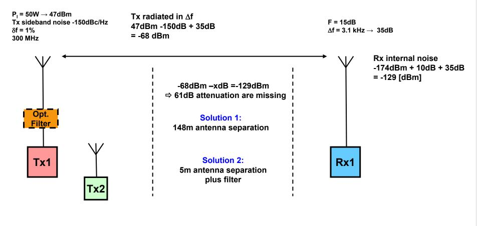
Desensitization of 3 db happens, if Tx noise and Rx noise at Rx input are equal
