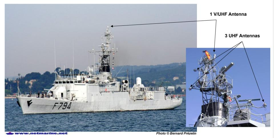
Example for a small installation V/UHF: 2 V/UHF radio lines Example for a large installation V/UHF:
